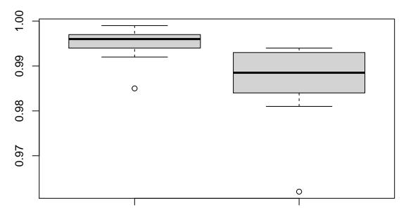
Ultrasonic Pulse Velocity Ratio with crack and without crack respectively
